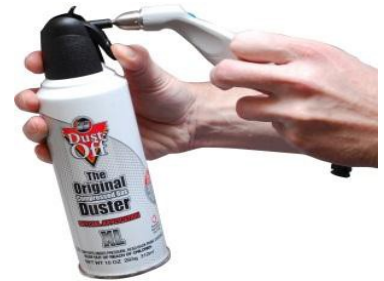
Compressed air being used to clean the tip of the AccuPen.
