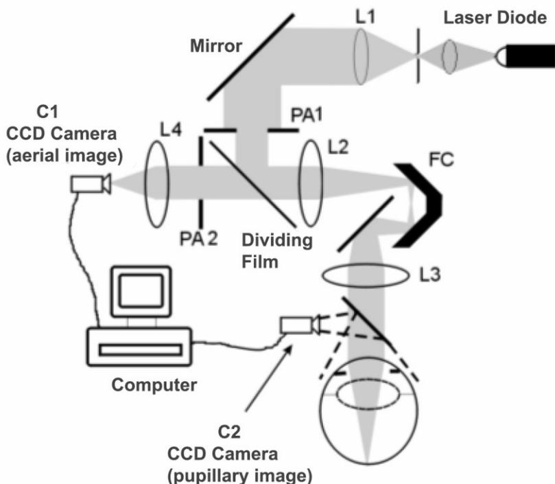
Figure 1. Double-pass diagram
